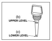
• If oil level is below the lower level line (c), refill with suitable oil (see table) to upper level line (b). Do not screw in the oil filler cap when checking oil level.
